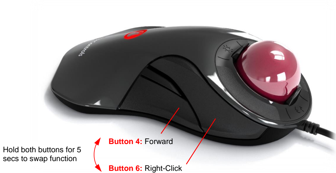
Figure 7: Right/Forward Button Configuration***
