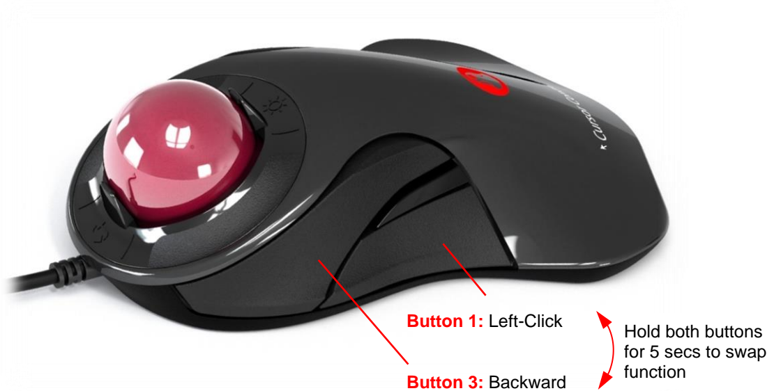
Figure 6: Left/Backward Button Configuration***
